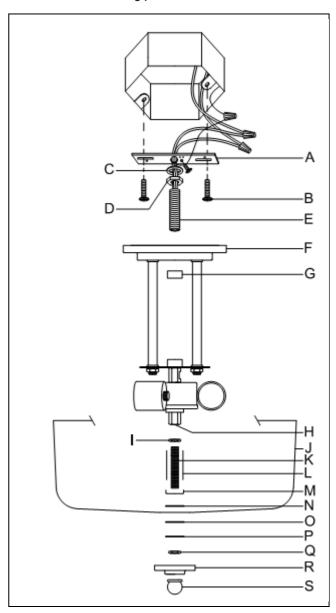
Line art shown may not exactly match the fixture enclosed. However, the installations do apply to this fixture. ITEM NO:414SF
