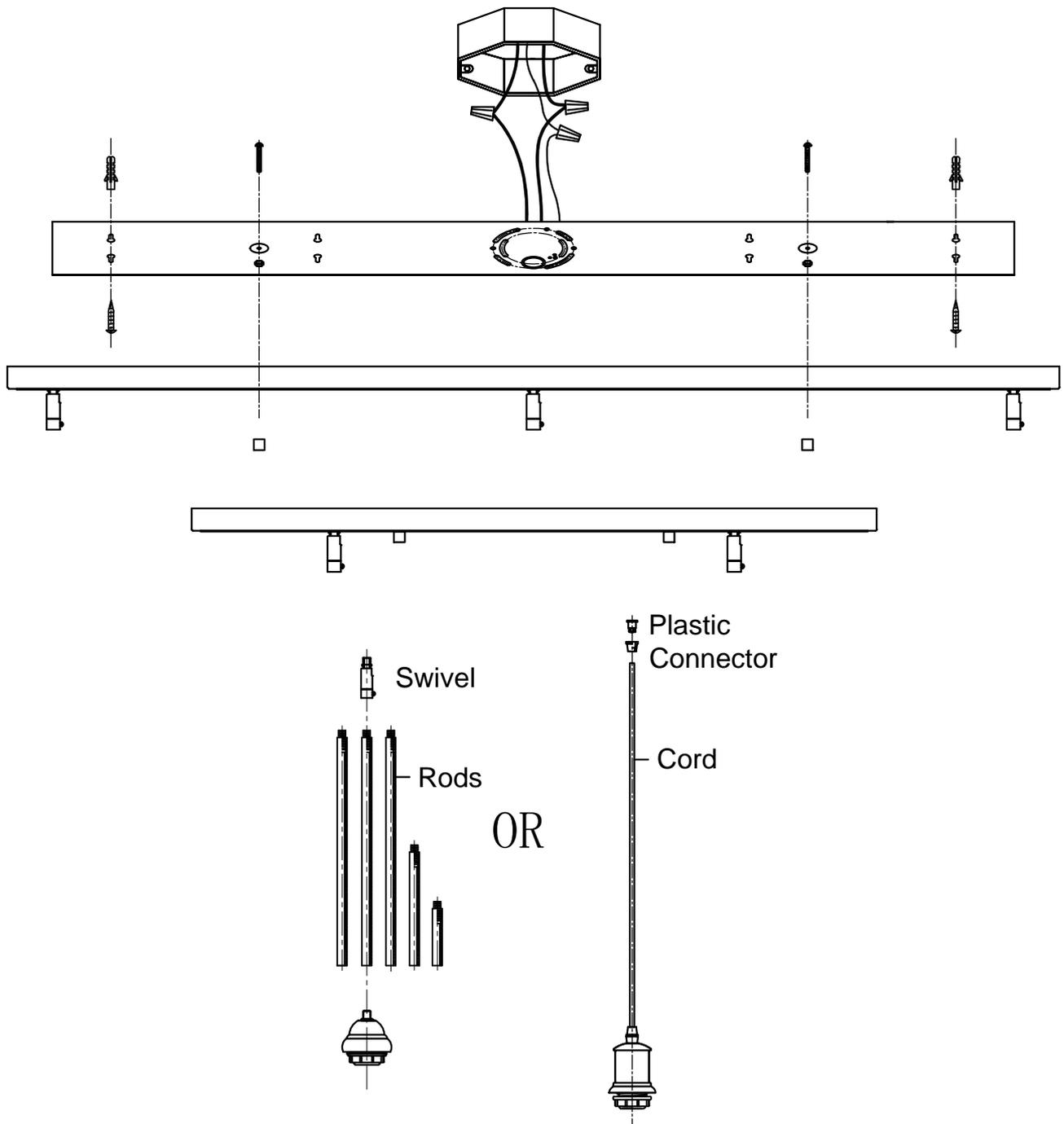
Rod mount fixture: Use the swivel included or the swivel from your fixture kits. Do not use plastic connectors.
